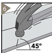
The last rows will not allow the use of the stapler. Manual nailing has to be done on the tongue. Pre-drill pilot holes at 45° and drive finishing nail.
