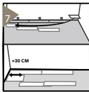
When starting the next row, always make sure to stagger the end joints by at least 12 in (30 cm). Try to use cut piece from previous row to start new row.
