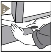
Lay a loose board upside down as a proper height guide against the door jamb. Cut the bottom of the frame off, leaving the required expansion gap allowance.
