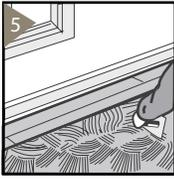
Lay the first row of starter boards along the chalk line/straight edge. Starting from the left corner, secure the boards into position with tongue-side facing the wall.
