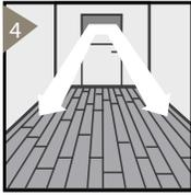
Boards shall run lengthwise against the longest wall. When possible try to run floor boards parallel to incoming sunlight or main light source. T-molding is required for rooms exceeding 1,080 sq ft (100 sq m).
