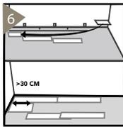
On starting the next row, always make sure to stagger the end joints by at least 12 in (30 cm). Try to use cut piece from previous row to start new row.
